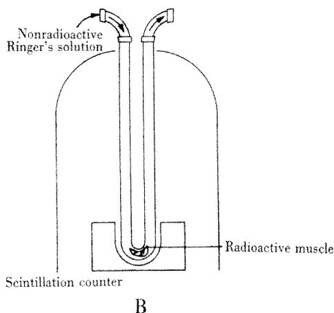
FIGURE 13. The U-tube,  $\gamma$ -scintillation counter assembly of Ling-Schmolinski for the study of  $^{22}\text{Na}$ - $^{24}\text{Na}$ - (and other  $\gamma$ -emitting radio-isotope-) labelled  $\text{Na}^+$  efflux rate studies of single and multiple frog muscle cells. (from Ling 1962, in his Figure 8-5 on page 198)
